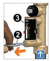
C. While holding the bypass valve open, use a wrench to turn the valve control stem (4) to adjust the flow rate slowly. The resulting flow rate is indicated by the metal ball (5) that slides up and down inside a transparent channel (6) marked by a graduated scale in gpm.
