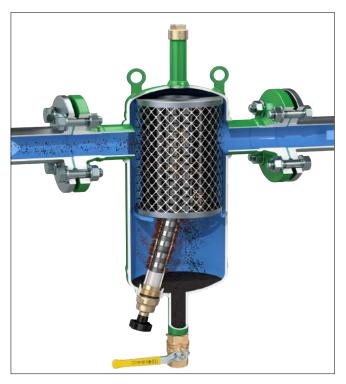
To purge the debris, the flexible magnetic stack is removed from the brass dry-well and, even while the system is still running, the drain valve is opened. Aided by the system pressure, the dirt and magnetite flushes out quickly and effectively. DIRTMAG® magnetic dirt separators accomplish 2½ times the ferrous impurities removal performance of standard dirt separators, delivering up to 100% elimination efficiency.
