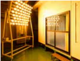
An actual air conditioner is operated in a test room that simulates a standard living room. The test makes it possible to confirm optimum performance level under ever-changing conditions.
