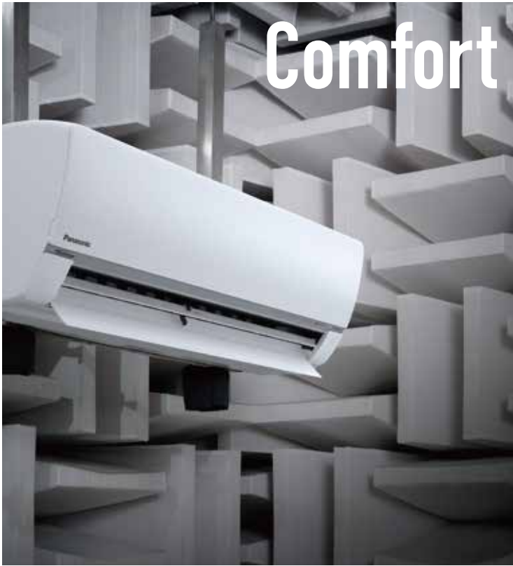
An actual air conditioner is operated in a test room that simulates a standard living room. The test makes it possible to confirm optimum performance level under ever-changing conditions.
